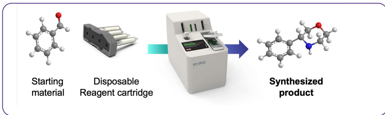
Figure 1. With ready-to-use automated synthesis platforms, chemists can conduct organic synthesis reactions within a contained system. Synple relies on reaction-specific disposable reagent cartridges to produce desired synthesis products. 4
